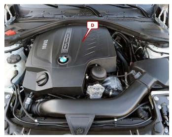
Open the engine hood. Remove the engine cover (D).
