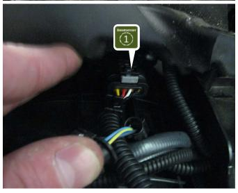
Localise the top right area from the engine compartment. The 4-pin manifold pressure sensor is located at the intake manifold after throttle valve. Disconnect the plug by open the locking lever and connect the correct boost pressure adapter in between.
