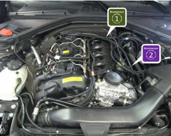
Connect the system to these three sensors: Intake manifold pressure sensor after throttle body, boost pressure sensor before throttle body of the engine.
