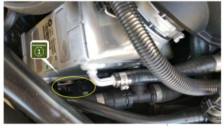
Localise the boost pressure sensor at the intercooler.Be Prepare sersors are in tight spot
