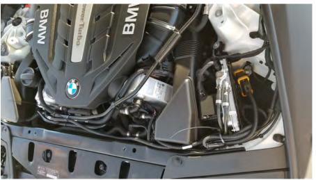
Route the harness and zip tie,Locate the ChipWerke in Cooler spot.
