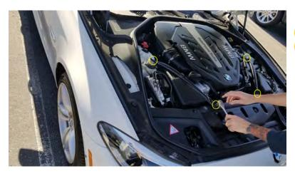
Go Ahead and remove the forward Support bars for easy access
