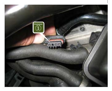
Disconnect the boost pressure sensor connector by unlocking the locking lever from the boost pressure sensor. Connect the adapter cable connection to these sensor. Do the same procedure on the other side.
